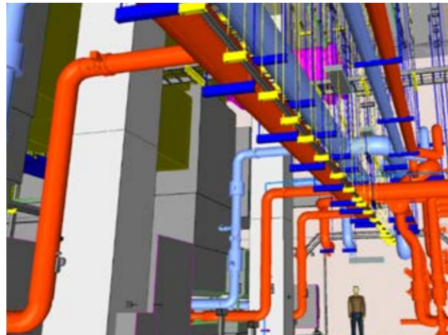
A beneficiary of the PSG in the 3D Modelling, Immersive Visualisation & Analysis category. The system facilitates clash detection, installation sequence and maintainability studies of Mechanical, Electrical and Plumbing Systems (MEP) services, such as in a plant room.
