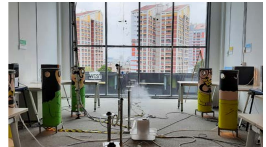
A test set-up in BCA's SkyLab replicating six occupants with sensible and latent heat load with CO 2 simulating respiration.
